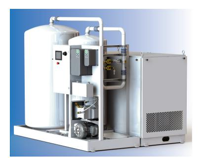
All units are fitted with a programmable logic controller (PLC) and a variable frequency drive (VFD) for the main blower motor. This feature gives the highest possible efficiency and also gives a linear power demand on *turn down*. When using 50% of the capacity of the machine, only 50% of the energy is required.
